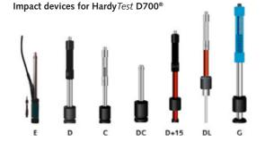
Impact device D: Universal device for most hardness requirements
